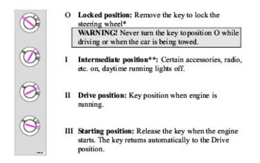
A chime will sound if the key is left in the ignition and the driver's door is opened. \* The gear selector must be in the (P)ark position.
